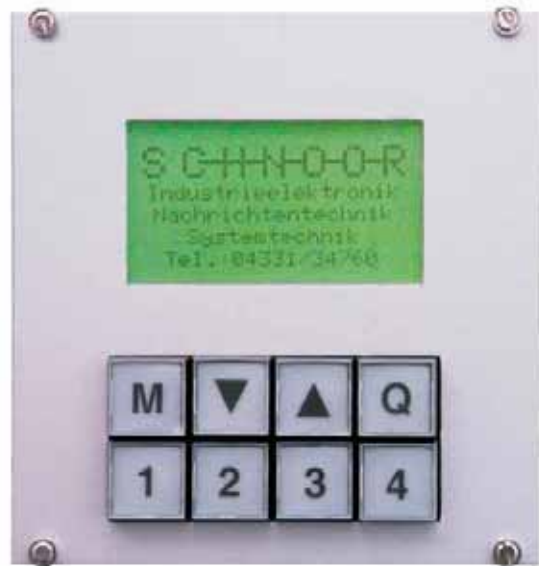
The monitoring unit WSDP can be integrated in 19" racks
